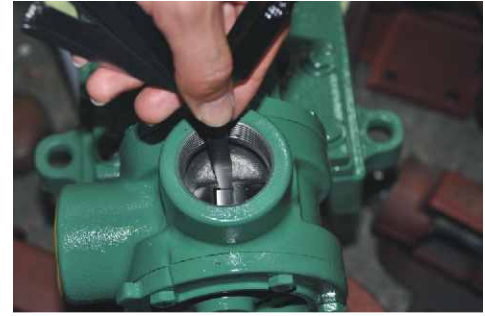
Figure 32: Checking the axial clearance with air gap gauge (feeler gauge).
