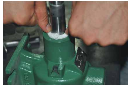
Figure 19: Repacking with hook tool and packing new rings.
