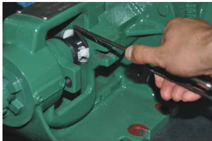
Figure 19: Repacking with hook tool and packing new rings.
