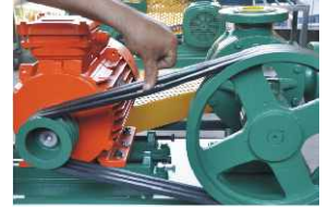
Figure 9: Belt tension adjustment
