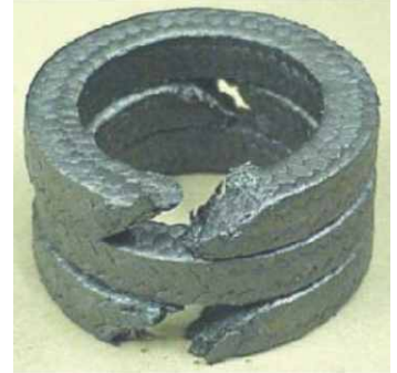
Figure 20: Packing Gland Rings
