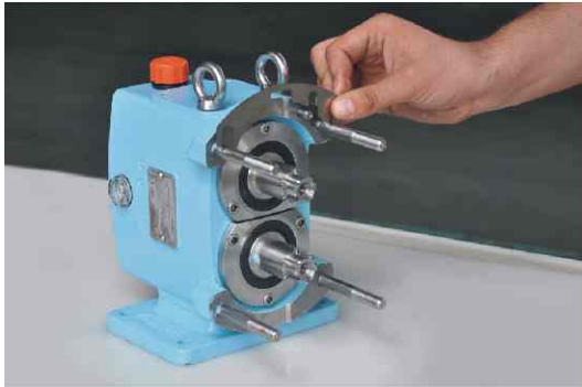
Figure 21: Disassembling the shim plates.
