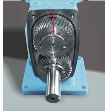
Figure 32: The locking tab of the bearing washer.
