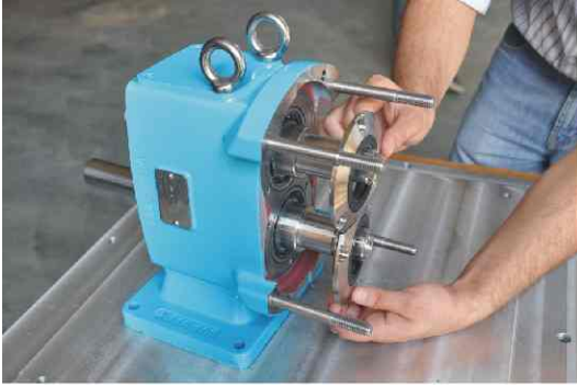
Figure 34: Disassembling the rear cover oil seal of the gearbox.
