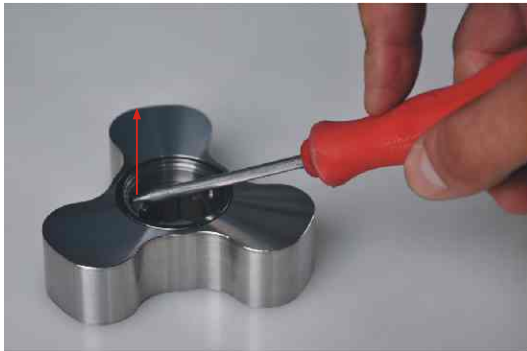
Figure 23: Using screwdriver for the ring of mechanical seal.
