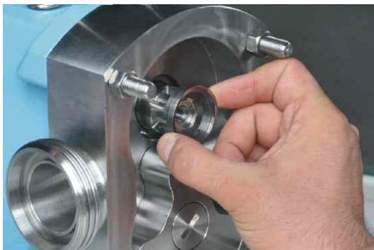
Figure 17: Disassembling the ring of mechanical seal on the pump.
