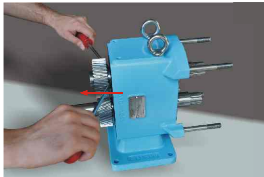
Figure 33: Disassembling the gears.
