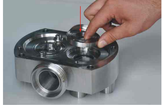
Figure 26: Assembling the case of mechanical seal.
