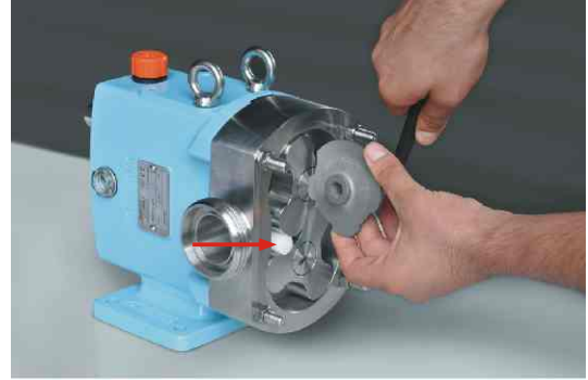
Figure 14: Using the special tool for rotor bolts.
