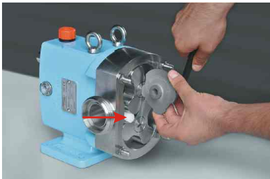
Figure 29: Assembling rotor bolts.
