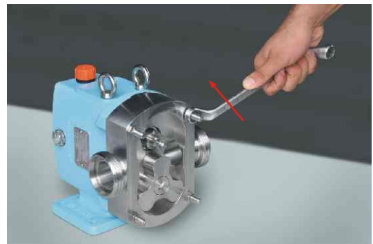
Figure 18: Disassembling the housing bolts.
