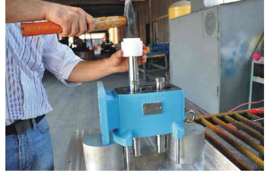
Figure 35: Disassembling the drive and idle shafts.
