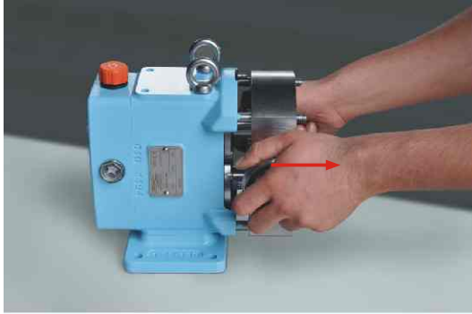
Figure 19: Disassembling the housing.
