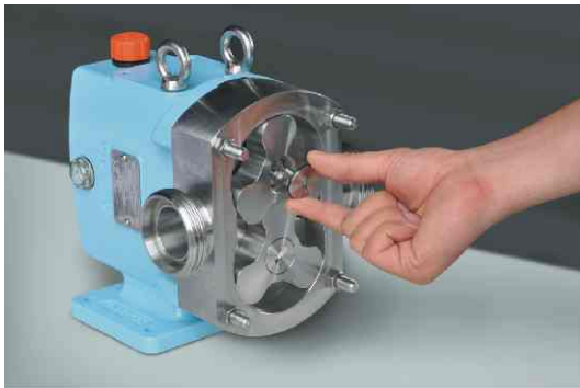
Figure 15: Disassembling rotor bolts.
