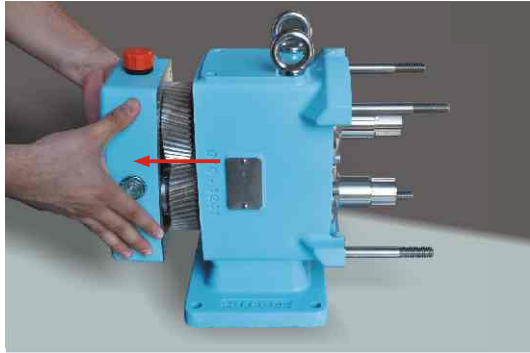
Figure 31: Disassembling the rear cover of the gearbox.
