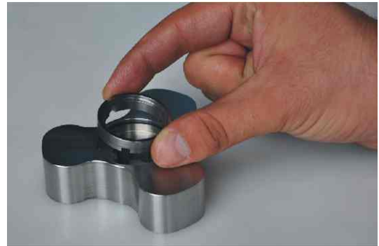
Figure 24: Assembling the face of mechanical seal on the rotor.
