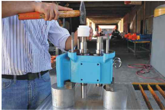
Figure 36: Assembling the drive and idle shafts.
