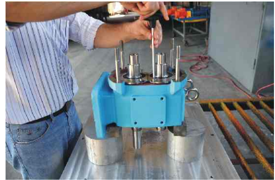
Figure 37: Assembling the lubricating cover of the gearbox.
