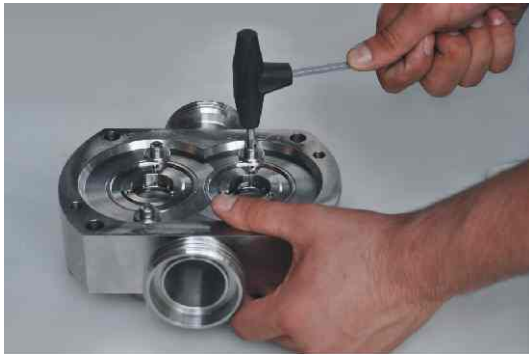
Figure 27: Tightening the case bolts of mechanical seal.
