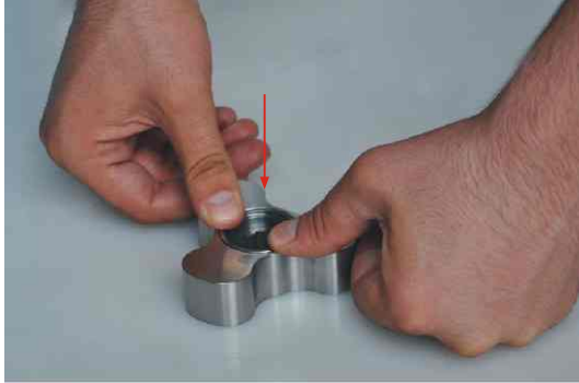
Figure 25: Assembling the face of mechanical seal on the rotor.
