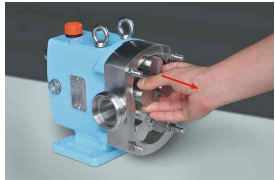
Figure 16: Disassembling the lobes.
