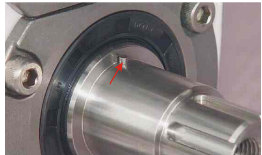
Figure 30: Fixing the pin of double mechanical seal.
