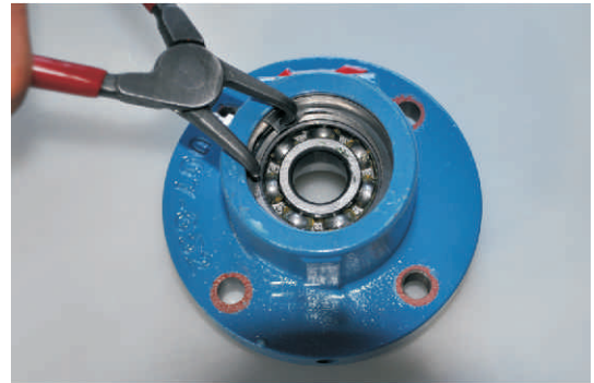
Figure 27: Shows extracting the inner snap ring by using plier.
