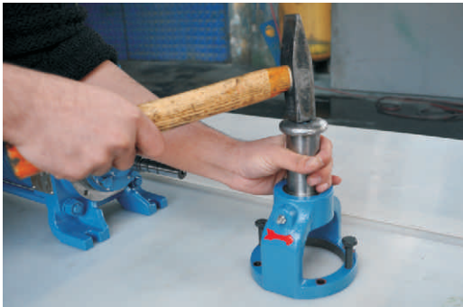
Figure 52: Shows placing the bearing into casing.
