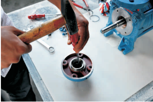
Figure 28: Shows extracting the ball bearing from mechanical seal casing.
