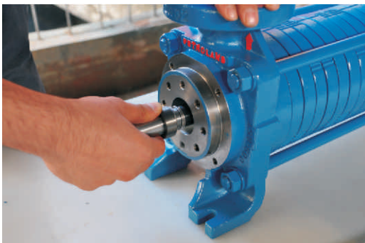
Figure 54: Shows placing the rotating seal on the shaft.
