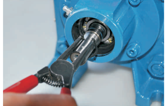
Figure 21: Shows extracting the bearing snap ring by using plier
