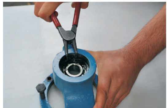
Figure 49: Shows extracting the inner snap ring by using plier.
