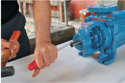
Figure 40: Shows replacing the key by using screwdriver and hammer.
