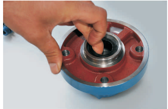
Figure 25: Shows pulling the stationary face from mechanical seal casing.
