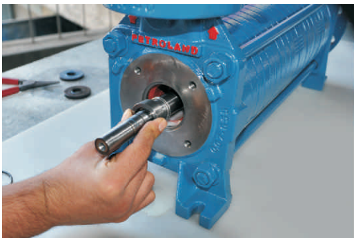
Figure 32: Shows placing the rotating seal on the shaft.
