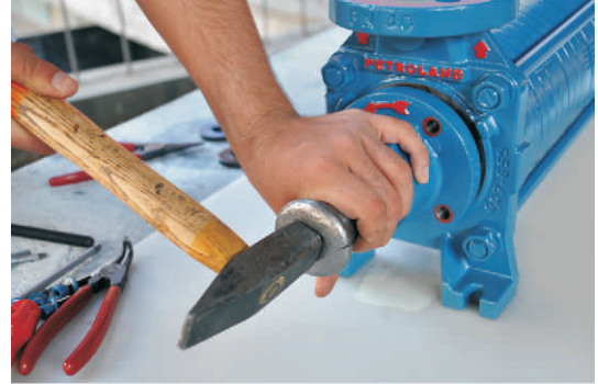
Figure 35: Shows fixing the mechanical seal face onto discharge casing.
