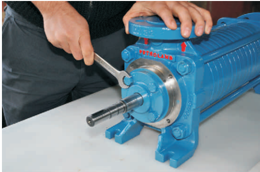
Figure 46: Shows untightening the screws of mechanical seal casing.
