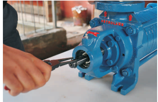
Figure 59: Shows fixing snap ring onto shaft
