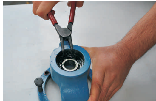
Figure 53: Shows fixing the inner snap ring by using plier.
