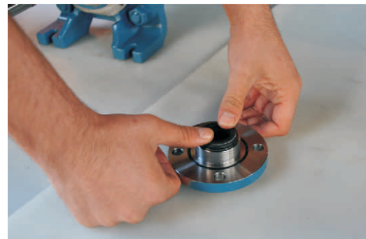
Figure 55: Shows placing the stationary face into mechanical seal casing.
