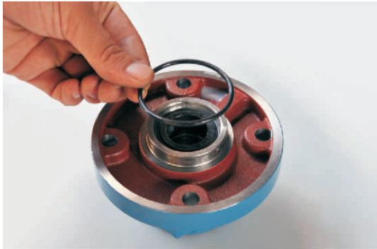
Figure 24: Shows removing the o-ring on mechanical seal casing.
