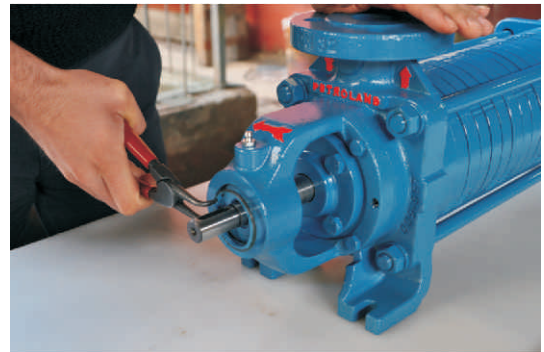
Figure 61: Shows fixing the snap ring of lip seal.
