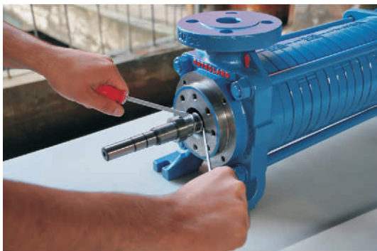
Figure 48: Shows pulling the rotating face and its spring
