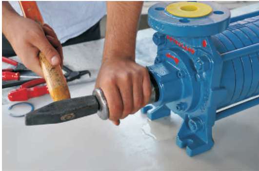
Figure 38: Shows fixing the lip seal into mechanical seal casing.
