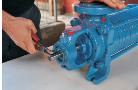
Figure 41: Shows extracting the inner snap ring by using plier.
