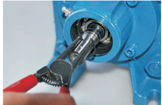
Figure 37: Shows fixing snap ring onto shaft
