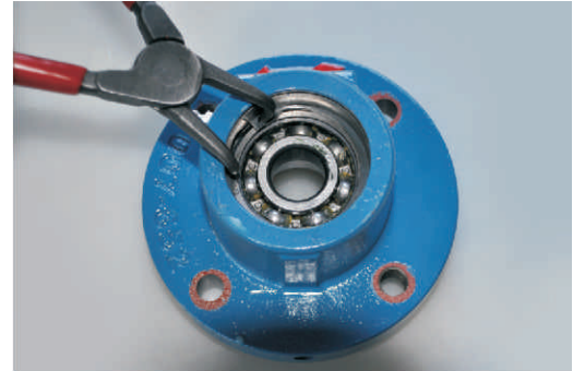
Figure 31: Shows fixing the inner snap ring by using plier.
