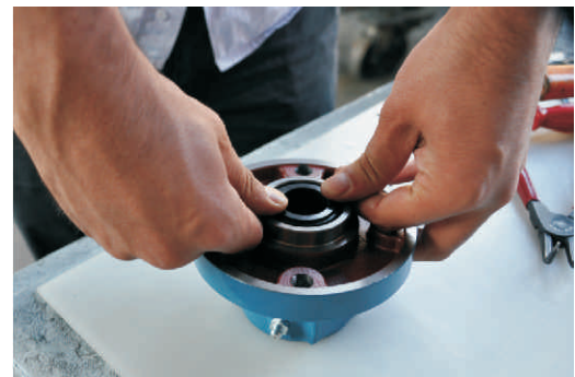
Figure 33: Shows placing the stationary face into mechanical seal casing.
