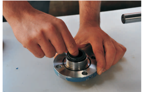
Figure 47: Shows pulling the stationary face from mechanical seal casing.
