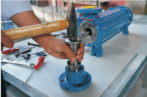
Figure 30: Shows placing the bearing into mechanical seal casing.
