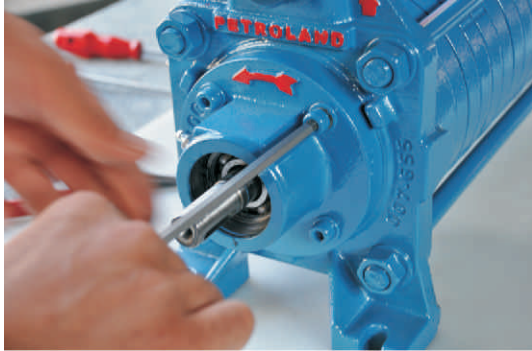
Figure 22: Shows removing the screws by using allen wrench.
