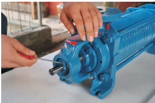
Figure 42: Shows extracting the lip seal by using screwdriver.
