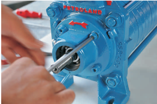
Figure 36: Shows tightening the screws by using allen wrench.
