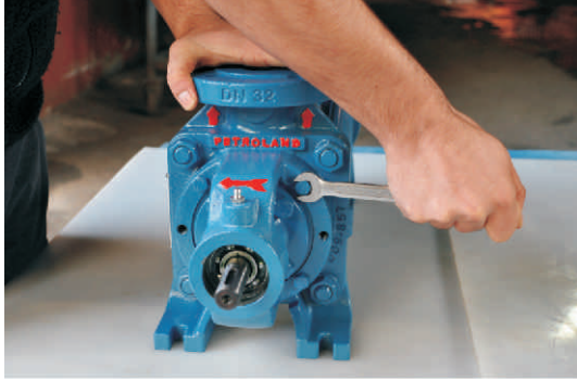
Figure 44: Shows removing the screws by using allen wrench.
