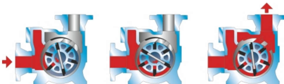
Working Principle of Petroland PV Series Pumps
