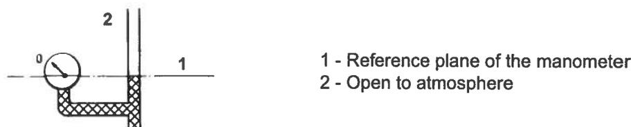
Figure I.1 — Arrangement for determination of reference plane of spring pressure gauges
