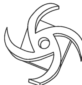
Figure 1.3.4.7 — Open impeller
