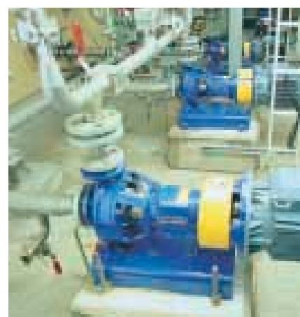
Regarding smaller motors, it is an advantage if the motor is flanged directly against the bearing assembly.
