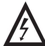
Safety sign according to DIN 4844-W8
