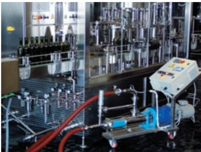
The product is fed delicately without sudden starts and stops but with pre-established accelerations and decelerations, avoiding hammering and sudden pressure variations. The microprocessor means that the signal sent by the detectors can be received and modified, according to the parameters set by the operator.
